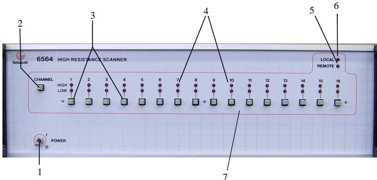
**Figure 3-1 Front Panel Guildline Model 6564**
