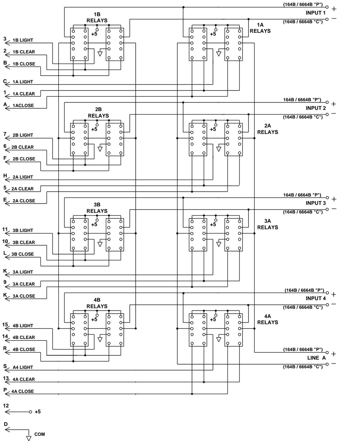
RELAY CIRCUIT BOARD, Connection for 2 Amp Relays
