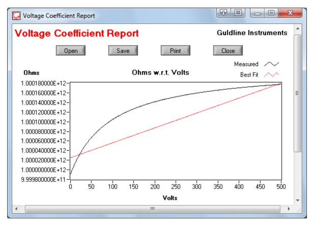
The Voltage Coefficient report window is a summary of many tests taken at different voltages. The average values of each test are plotted on a graph to show the voltage curve. From this curve, the best fit line is used to calculate the voltage coefficient. This report also contains the environmental conditions, test conductor and calculations for the test. From this report you can view the current test, open and save report files, as well as print out a hard copy.
