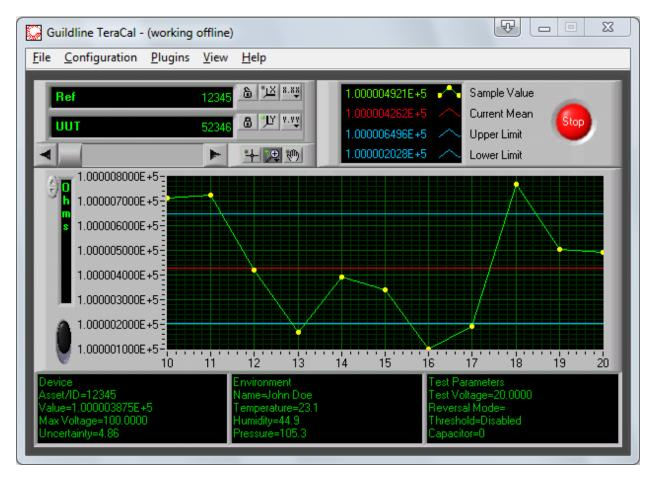
In the main window, there is a series of indicators and controls to setup and observe the measurement process. There is also a menu bar to access most of the functions and features of TeraCal.
