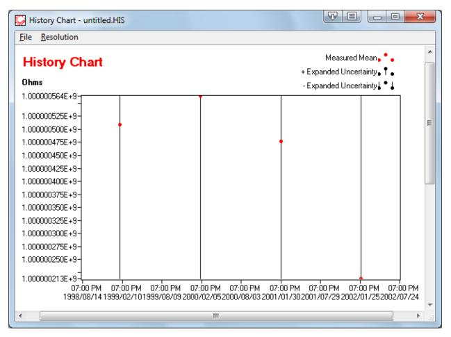
The History Chart window is similar to the Test Overview window, except that the viewer is made to open and create "\*.HIS" history files. History files are cumulated test "\*.TES" file data grouped into one file for the purpose of analyzing many measurements on the same resistor.
