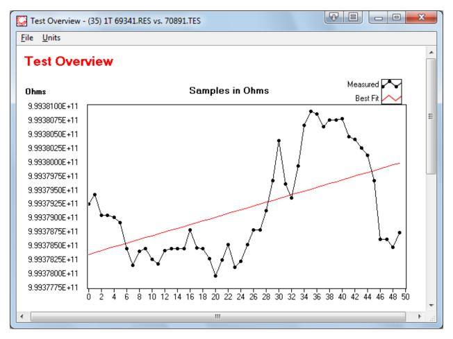
The Test Overview window is where you can open and edit saved test data. This window will complete a data analysis of the opened test file and display a graph with the best-fit curve; as well as mean, standard deviation and uncertainty calculations. These are all displayed in a clean, organized report format, which can be printed out.
