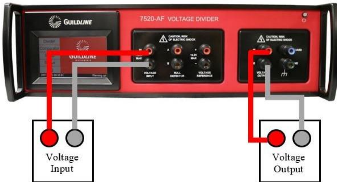
Figure 3-4: Model 7520 Connections for Operation as a Voltage Divider
