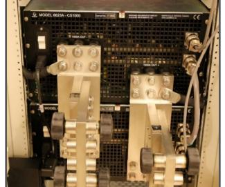
output current is 0.1% or 1000 ppm versus as low as 5 ppm for Guildline's 6623A-PCS.
