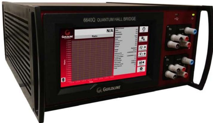
**GUILDLINE INSTRUMENTS 6640Q QUANTUM HALL RESISTANCE (QHR) BRIDGE** has been completely redesigned to provide better uncertainties and more operational capability. The 6640Q Quantum Bridge incorporates many patented new design and measurement technologies to provide a Precision Resistance Bridge operating at room temperature that will scale from the Quantum Hall resistance value of 12906.4035  $\Omega$  to nominal resistance values of 0.1  $\Omega$  to 100 k $\Omega$ .
